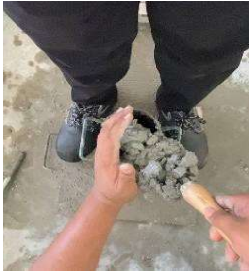
Figure 4: Cone filled with concrete
