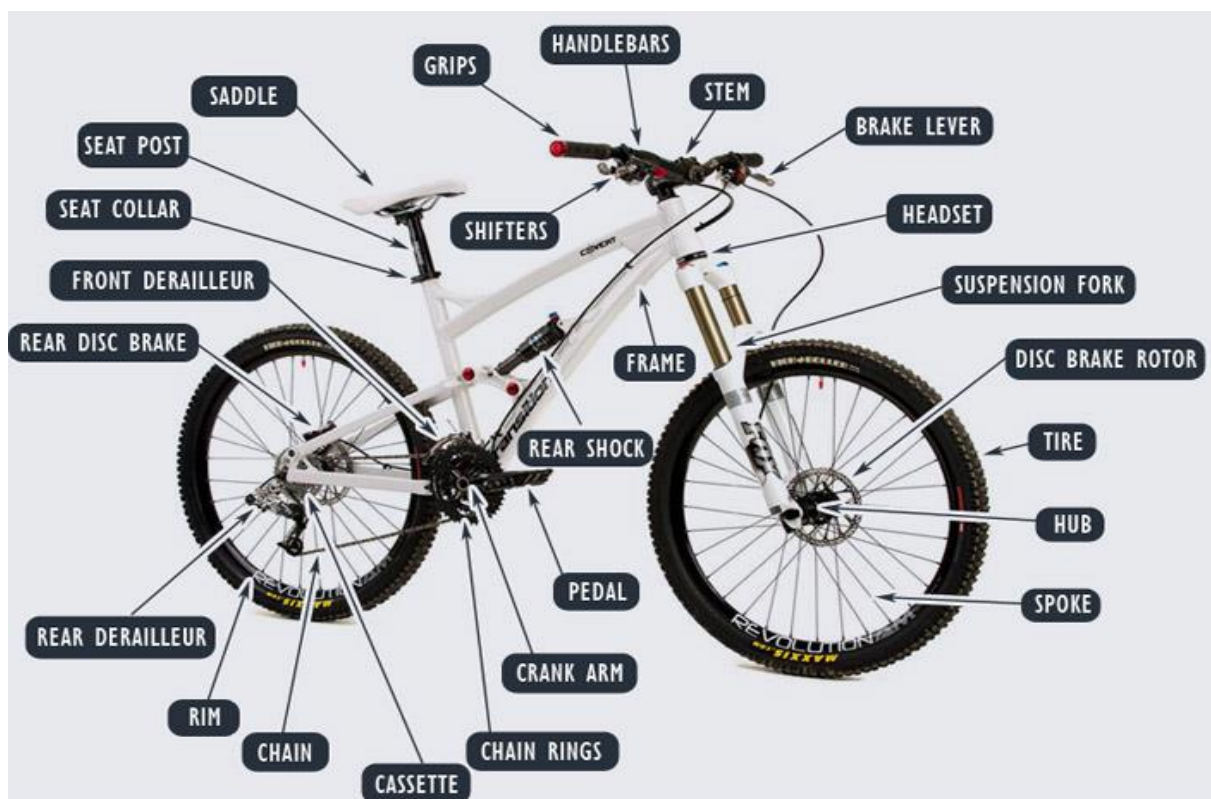
Gambar : Anatomi Basikal Mountain Bike Full Suspension
